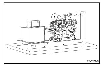
Figure 3-2 Single-Pad Mounting
